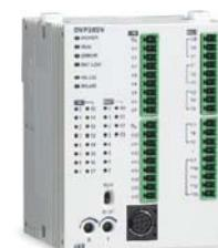
SV series satisfies all kinds of applications. It supports simple I/O control and high-grade 4-axis motion control, as well as all kinds of industrial network modules. Left side is extendable by special extension modules and right side by general extension module, totaling 16 extension modules extendable to DVP-SV.
